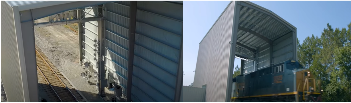
Picture reference here (Left: the system with cameras lined 360 degrees; Right: the train passing through)
